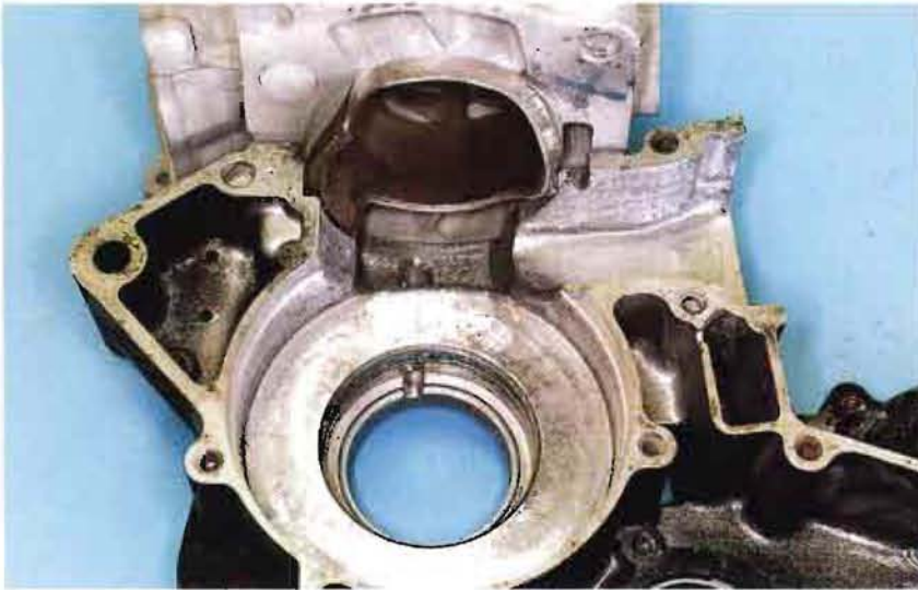
Case-reed engines can benefit from crankcase porting and cylinder matching more so than cylinder-reed engines. Case porting is a metal finishing task that serves to match the crankcase and cylinder transfer ports and polish surface imperfections.
