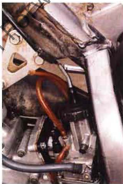
The number one cause of stuck throttle condition is a bad throttle cable. Improper routing caused this cable to fray above the carburetor. The cable should route through the center of the head-stay brackets.
