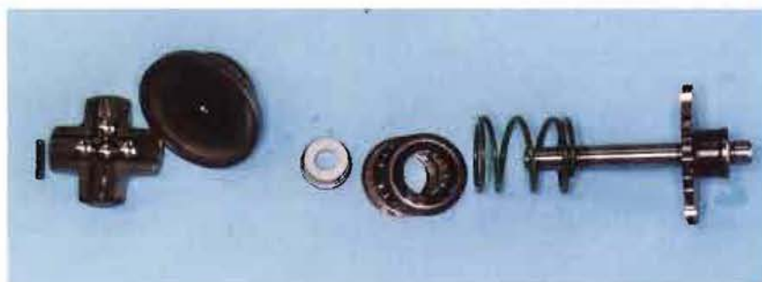
A centrifugal governor mechanism converts rotary motion from the crankshaft and turns it into linear motion to vary the exhaust port's effective stroke matched to rpm. The four steel balls travel in channels on a ramp. The higher the rpm, the farther the balls travel up the ramp, overcoming the force of the spring.
