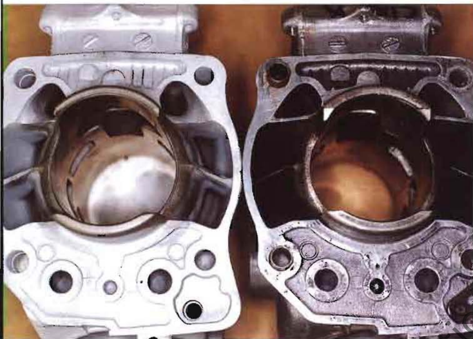
The cylinder on the left is ported and the cylinder on the right is stock. Porting is a metal machining operation that includes general smoothing and matching of the ports with port timing changes made at the intersection of the port windows and the cylinder bore.
