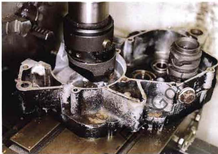
This crankcase is being bored on a milling machine. Because the crankshaft was stroked for a 2-mm offset, the area where the connecting rod swings past the crankcase must be bored 4 mm larger for the proper clearance.
