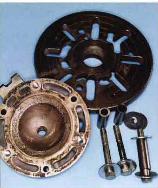
Cylinder heads with offset spark plug holes must be mounted to a face-plate for machining in a lathe. Three of the bolt holes are tapped to a 3/8-NC thread and spaced from the plate with wrist pins and washers.
